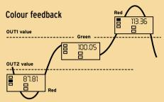
You can choose to have the display value in Red or Green. Both colours are available in one model. With these colours you can give an intuitive feedback of your process (applies only to models with outputs).
