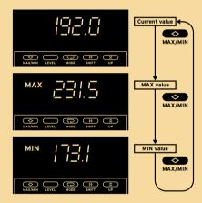
For daily process control of Maximum & Minimum process values you can directly read these values out by pressing the MAX/MIN button. Switching off the power supply resets the indicator.
