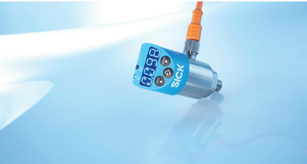
The pressure switch PBS is designed for pressure monitoring and measurement in liquid and gaseous media. It is pressure switch, transmitter and display in one and the same device. In its standard configuration it has two switching points (PNP or NPN). In addition, there are configurations available with one or two switching points and an analog output signal (4...20mA oder 0...10V).
