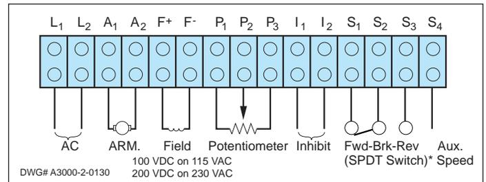
**Note:** Only 10 mA of current is switched. Any switch or relay may be used except a solid state type or a relay with capacitors or R-C networks (snubbers) across its contacts.
