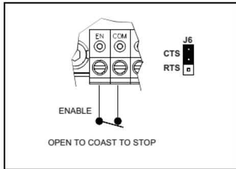
\*FWD Accel and REV Accel do not affect the stopping time when the enable circuit is opened.
