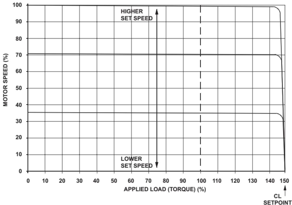
FIG. 7 – TORQUE CONTROL MODE (Linear)
