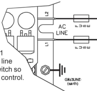
**A. AC Line** – Connect AC Line to terminals L1 and L2. (Be sure jumpers J1A and J1B are set to match the AC line voltage used.) (See table 5, p. 10.)
