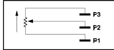
1. Remote Potentiometer – Connect remote potentiometer wires to terminals P1, P2 and P3, so that the "high" side of the potentiometer connects to P3, the "wiper" to P2 and the "low" side to P1. (See figure 11.)
