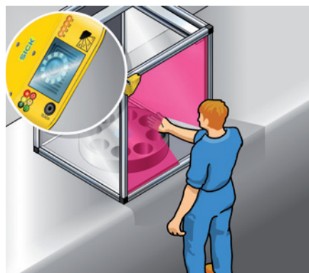
Hazardous point protection on a semi-automatic assembly machine.
